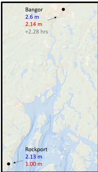
Figure 1. October 30th, 2017 storm surge map for the Penobscot River. Site locations are in Rockport and Bangor. Blue text values are peak storm tide (tides + storm surge), red text values are peak storm surge, grey values denote time for surge to travel from Rockport to Bangor.
